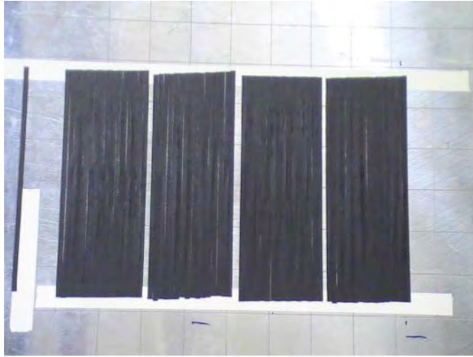
Figure 1 – Four test patches of carbon fiber tow. Each is 16 tows wide.
